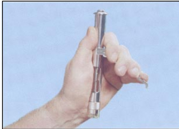
Fold the charging arm over completely to load
